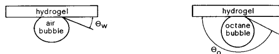
Fig. 2. Schematic drawing, indicating contact angle measurements on a hydrogel (e.g. mucosa or polymer) using either an octane drop or an air bubble, in an aqueous medium. The surfaces of interest are facing downward.
